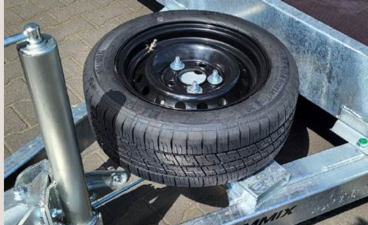
Spare wheel on box section
